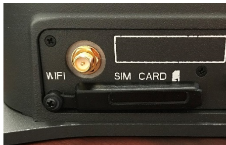
Figure 2-11 Secure the SIM Card Cover
