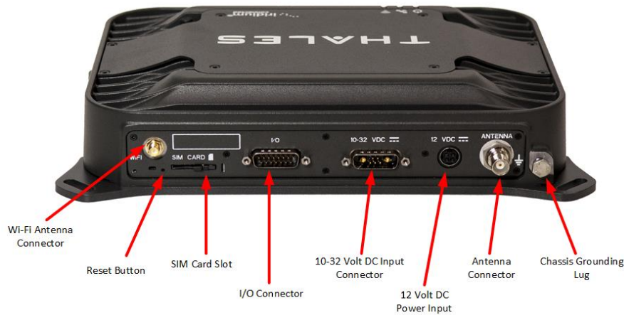
Figure 1-5 Below Deck Unit (BDU) Back Panel Detail
