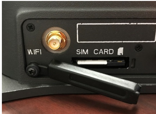
Figure 2-9 SIM Card with Cover Opened
