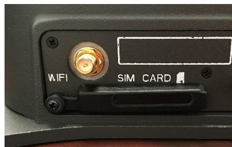
Figure 2-7 Secure the SIM Card Cover
