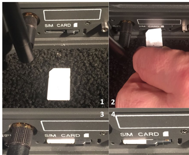
Figure 2-6 Installing SIM Card and Engaging the Lock
