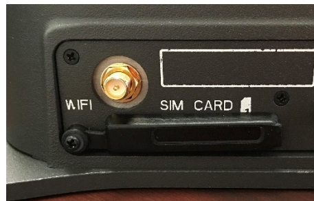
Figure 3-5 Secure the SIM Card Cover
