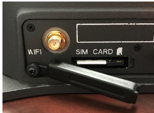
Figure 3-3 SIM Card with Cover Opened
