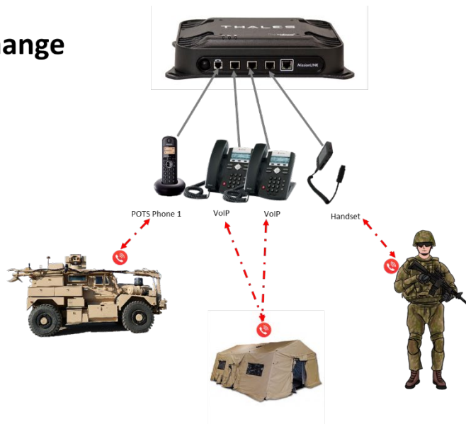
Figure 2-2 Local Communications via PBX Functionality
