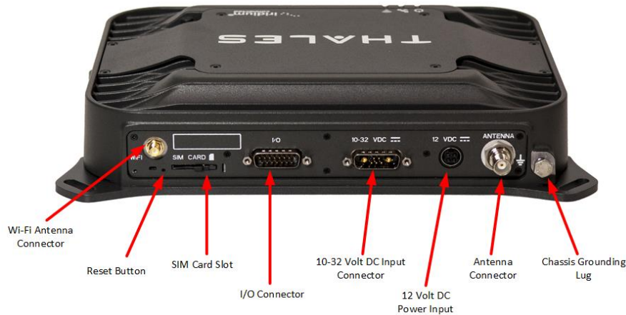
Figure 2-7 Below Deck Unit (BDU) Back Panel Detail
