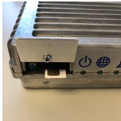
Figure 31: Installing the SIM card
