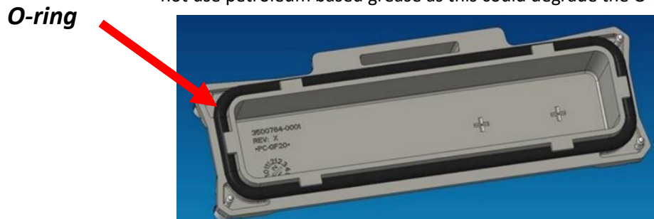
Figure 42: End Cap O-ring
